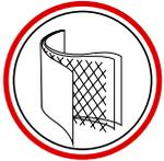
**Scrim Reinforcement:** When you need plastic sheeting to be light weight but extremely puncture and tear resistant you should consider something with scrim reinforcement. The polyester scrim is sandwiched between the layers of polyethylene to enhance the durability of the film.
