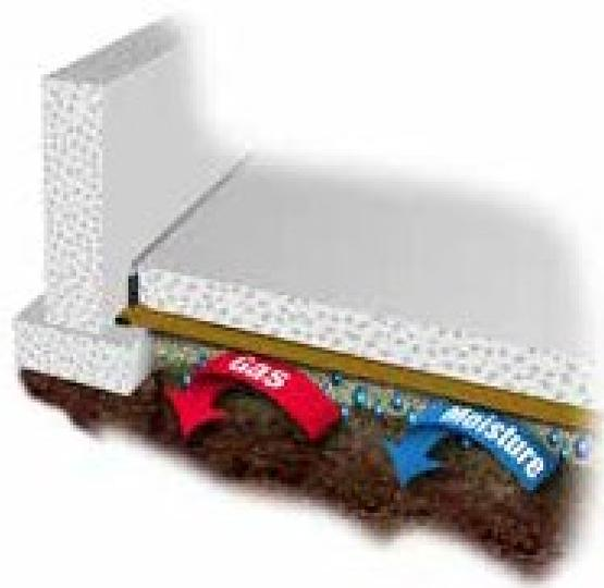
Note: Please refer to ASTM E 1643 (Standard Practice for Installation of Water Vapor Retarders Used in Contact with Earth or Granular Fill Under Concrete Slabs) and the appendixes that accompany this standard to provide additional installation information. Please follow all architectural drawings/instructions and conform to all applicable local, state and federal regulations and laws pertaining to residential and commercial building construction.
