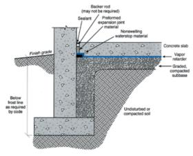
Figure 8-3. Nonreinforced concrete slab on ground.
