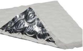
TempShield® Double Bubble White/Foil in a concrete slab application is two-fold; first, it acts as a vapor retarder and second, it provides a thermal break. The thermal resistance of TempShield® product under concrete is based on testing done on a calibrated hotplate using ASTM 518 test procedures.
