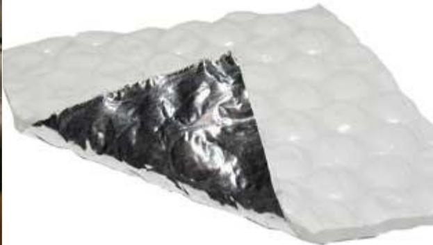
The purpose for installing TempShield® Single Bubble White/Foil in a concrete slab application is two-fold; first, it acts as a vapor retarder and second, it provides a thermal break. The thermal resistance of TempShield® product under concrete is based on testing done on a calibrated hotplate using ASTM 518 test procedures.
