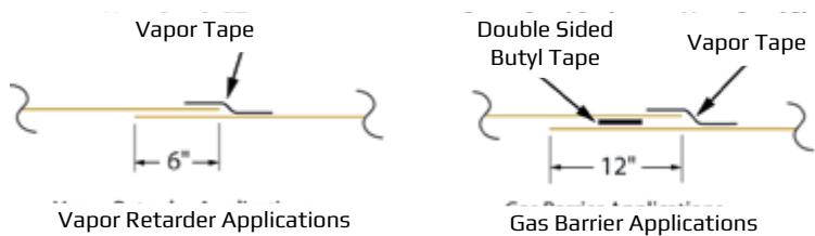
Fig. 2: VaporBlock Plus overlap joint sealing methods
