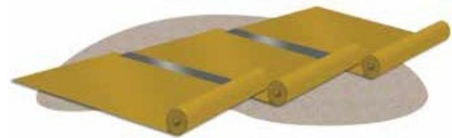
Fig. 1: VaporBlock Plus overlapping roll-out method
