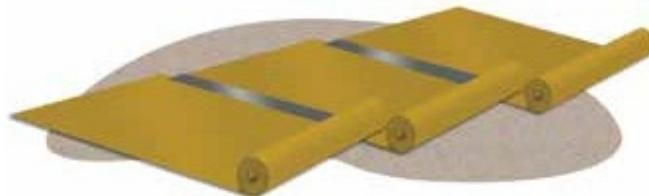
Fig. 1: VaporBlock Plus overlapping roll-out method
